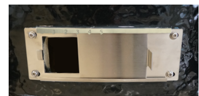
lower draft door at position 3
