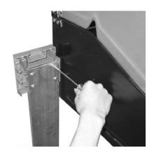
Secure the Legs (C8), (C9), (C10), (C11) to the Endcaps (C3), (C4) and the R/H Side Shelf (C6) using the Screws (D4).
