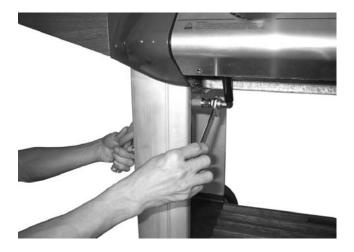
Connect the gas hose (if supplied) to the BBQ. Ensure the mating faces of the connection are clean and not damaged. Do not use any sealing tape, paste, or liquid on the joint. The nut must be tightened with the use of a spanner. Do not use force which may damage the assembly.
