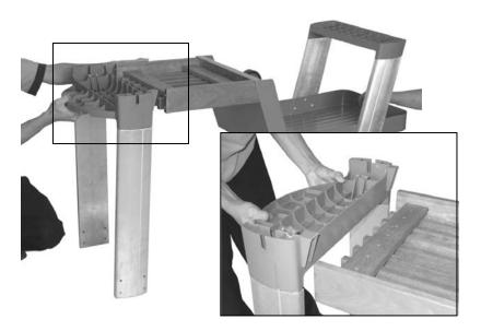
Align the Gas Bottle Holder (C14) with the Slat Assembly (C12).
