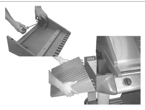
Attach the Side Shelf Hook (C22) to the L/H Side Shelf (C1) using the Screws (D5), Hook the side shelf to the endcaps.
